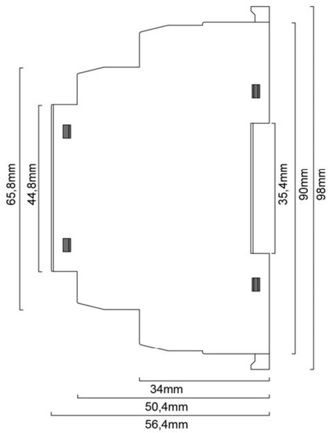
Geometry MC4LHS (din rail mounting)
